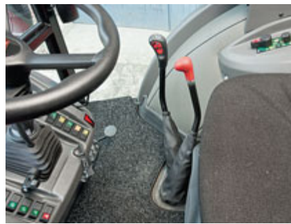
Red-handled lever operates the mechanical shuttle forward/reverser; the other tall lever shifts through the four main gears. Buttons control the three powershift steps.
