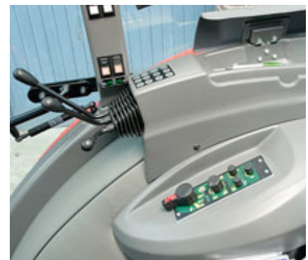
ELC operation is excellent. Only tester complaint was that the spool levers reside all the way over on the cab's B-post.
