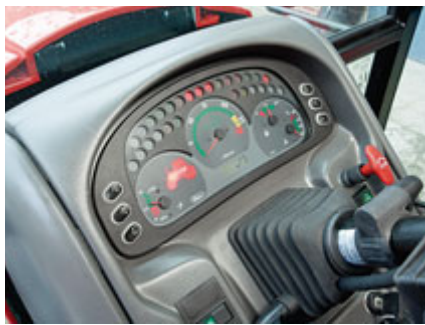
Dash controls are neatly grouped. Downers include the digital read-out being too small and the tractor having just the one display for ground speed, pto speed, hours etc.
