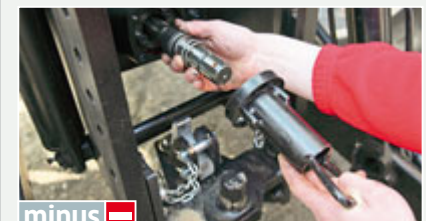
We had to turn the stub on our Dutch test tractor to alter the pto speed. Zetor UK says that, as an option, this job can now be done from the cab.
