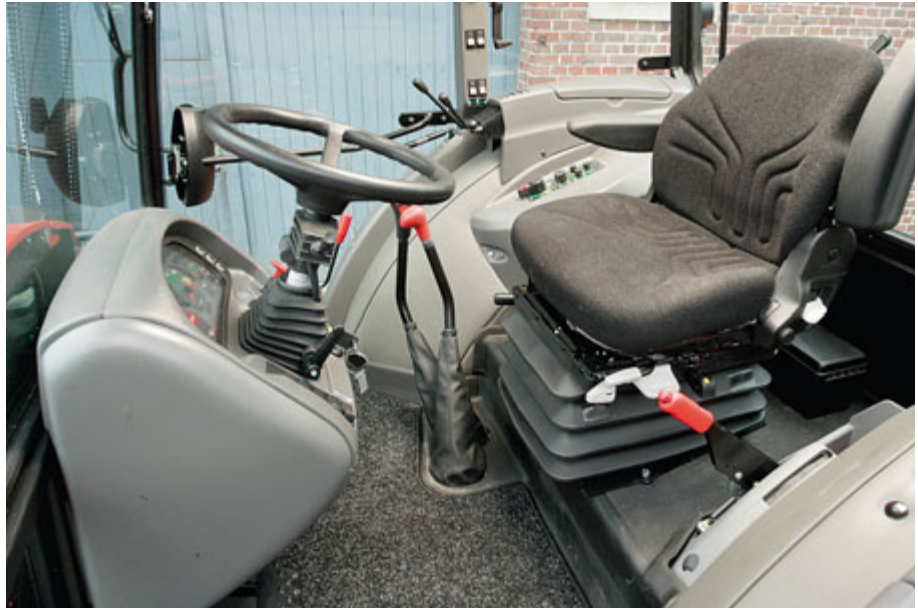
The large, air-suspended cab is workmanlike. Though the DLG recorded a noise level as high as 80.0dB(A), operators were pleased with the cab in practice. There are no fan vents in the roof.
