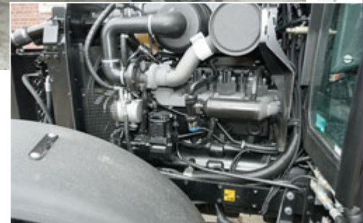
The new 16-valve engine proved powerful and economical on the test stand. The Stage IIIA compliant unit mixes new and old technology, incorporating cooled and external exhaust gas recirculation (inset), but still relying on a mechanical injection pump.
