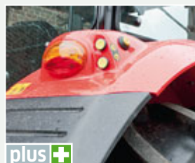
Our Dutch-supplied test tractor had mudguard-mounted controls for linkage and pto.
