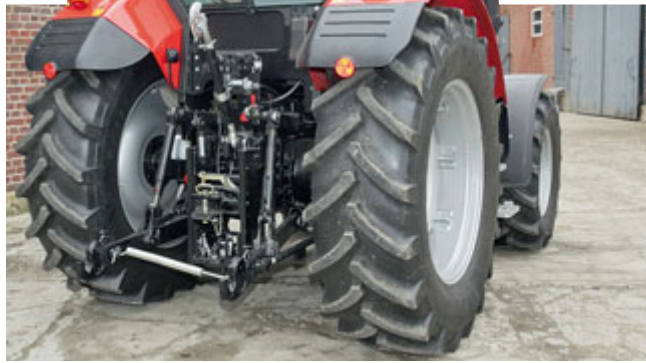
UK/Irish spec tractors come with a Dromone push-back hitch, while the ineffective stabilisers (right) can be replaced by Walterscheid options. Mudguards are scheduled for strengthening.
