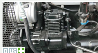
The standard compressor is flanged in place. It's a neat arrangement.
